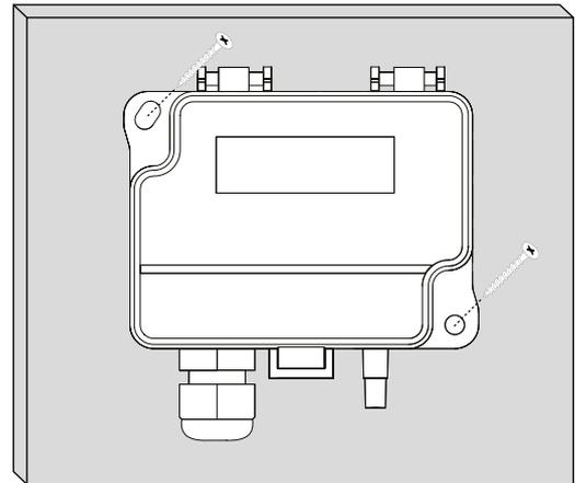
Figure 1b - Mounting orientation
